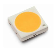
LUXEON 3030 2D is the first hot-color targeted mid power LED. Hot-color targeting ensures that the LEDs are within color target at application conditions—85°C. Using an industry standard packaging of 3.0mm x 3.0mm x 0.5mm and 6V surface-mount emitter solution, LUXEON 3030 2D comes in all ANSI CCTs and delivers the efficacy and reliability required for indoor illumination markets.
